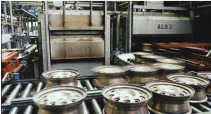
Aluminium industry: curing oven for wheel rims
